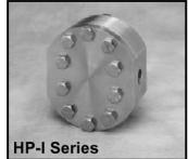
Flowdata flowmeters use two rotating impellers which are driven by the flowing liquid. Magnets imbedded in the impellers activate a non-intrusive sensor which generates a pulsed output signal. Each pulse represents a known volume of liquid that is captured between the lobes of the impellers. A "K-Factor" converts the pulses into engineering units for remote data collection and digital display.
